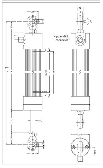
Important: all the data reported in the catalogue (linearity, lifetime, temperature coefficient) are valid for a sensor utilization as a ratiometric device with a max current across the cursor Ic  $\leq 0.1 \ \mu$ A.
