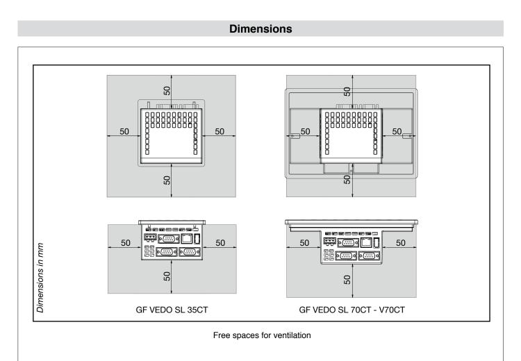
Attention: the temperature inside the compartment that houses the integrated Controller and Operator Panel must never exceed 50 °C.
