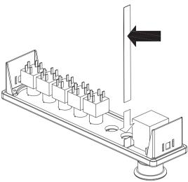
The card is inserted laterally from the left towards the right (seen from the rear, the keyboard has the slot at the top). The arrow shows the printed side of the card.
