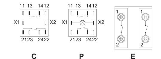
**Electromechanical component Features** Dim. Name Code Colour Туре Contacts ø mm Emergency "Mushroom" Stop ΡE Red head 40 2 NC: (1-2), (1-2) (push-pull) (E) 2 NO: (13-14), (23-24) P1 White Impulse Buttons (P) P2 Red command 1 Bulb: X1 (+24Vdc), P3 Green button X2 (0Vdc) С 2 positions (Latching) 1 NO: (13-14) 1 NC: (21-22) Key (C) Black 16,2 Emergency plug ΤE Black -22 \_ Plug Button T1,T2,T3,T4 Black 16,2 \_ \_ Key
