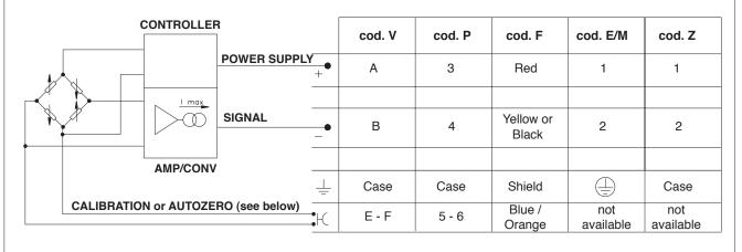
Option M: Magnetic Autozero Option E: External Autozero Activation of CALIBRATION function Activation of AUTOZERO function
