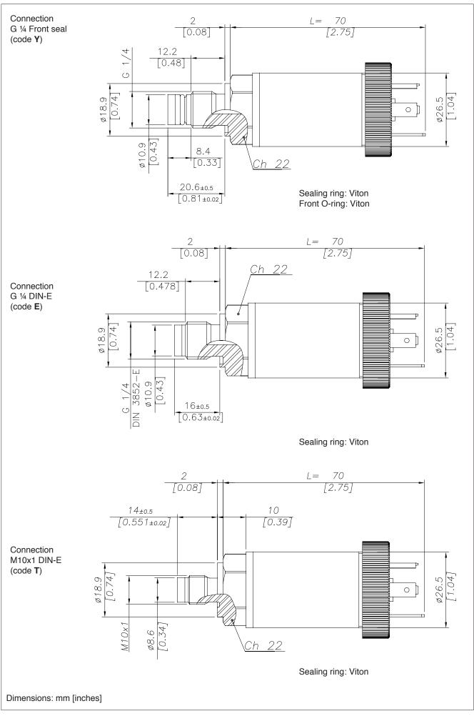
ATTENTION: for correct installation do not exceed 40Nm torque force
